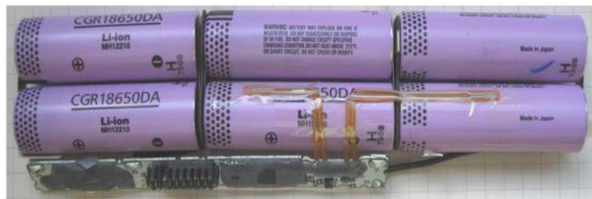
Figure 3.9: 3S2P Battery Setup
