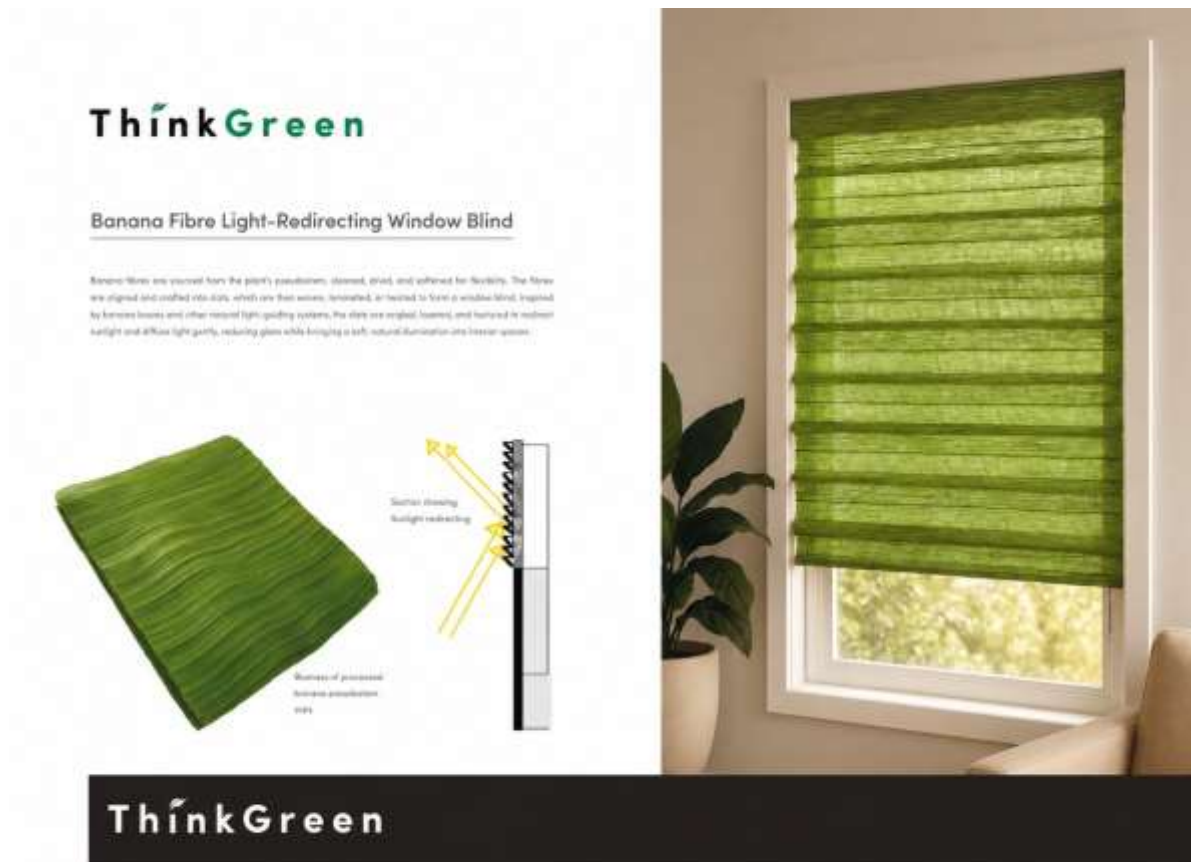
Figure 2: Prototype concept for the Banana Fibre Light-Redirecting Window Blind — showing processed pseudostem slat material (left), sectional diagram of sunlight redirection mechanism (centre), and interior render of installed blind (right). Model and rendering by the author.
